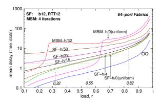
Fig. 7. Delay of well-behaved flows in the presence of hotspots.  $h/\bullet$  specifies the number of hotspots, e.g., h/4 corresponds to four hotspots. Bernoulli fixed-size cell arrivals; 64-port fabric, b=12 cells, RTT=12 cell-times (time-slots). Only the queueing delay is shown.
