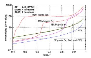
Fig. 6. Delay versus input load, for varying fabric sizes, N; buffer size b=12 cells, RTT=12 cell-times (time-slots). Uniform Bernoulli fixed-size cell arrivals. Only the queueing delay is shown.
