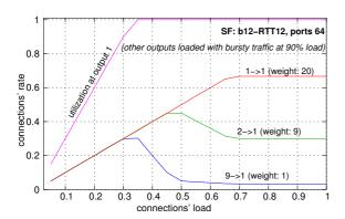
Fig. 9. Sophisticated output bandwidth allocation, using WRR/WFQ credit schedulers; 64-port fabric, *b*=12 segments, RTT=12 segment-times.
