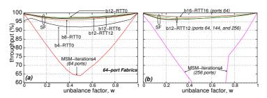
Fig. 5. Throughput under unbalanced traffic. 100% input load consisting of fixed-size cell Bernoulli arrivals. (a) 64-port fabric (N=64, M=8); (b) varying fabric sizes up to N=256. M=16.
