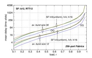
Fig. 8. Delay of well-behaved flows in the presence of hotspots, for varying burstiness factors. Bursty fixed-size cell arrivals; 256-port fabric, b=12 cells, RTT=12 cell-times (time-slots). Only the queueing delay is shown.
