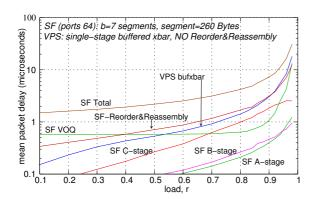
Fig. 11. Packet delay performance under variable-size packet arrivals, using variable-size multipacket segments; uniform Poisson packet arrivals on 10 Gbps input lines; b=7 (maximum-size) segments. Packet delay includes the request-grant delay, segment scheduling and propagation delays, as well as segment reordering and packet reassembly delays.
