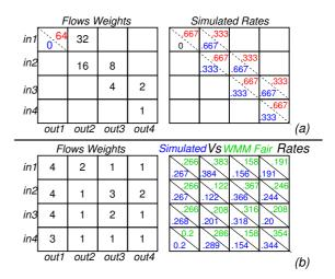
Fig. 10. Weighted max-min fair allocation of input and output port bandwidth, using WRR/WFQ schedulers; 4-port fabric, b=12 segments, RTT=12 segment-times.
