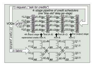
Fig. 2. pipelined buffer scheduling in a  $4\times 4$ , three-stage non-blocking fabric.
