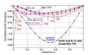
Fig. 7. Throughput under unbalanced traffic for varying buffer size, B, and varying threshold values, TH, using common-order round-robin credit scheduling; N=32; Bernoulli arrivals.
