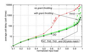
Fig. 5. Performance under bursty traffic, for different grant throttling thresholds, TH; N=32, B=12; average burst length 12 cells.
