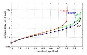
Fig. 10. Performance under diagonal traffic for OQ, iSLIP with 4 iterations, buffered crossbar with 1-cell crosspoint buffers, and for the switch we propose in this paper with B=12, TH=5, and desynchronized clock credit schedulers; N=32: Bernoulli arrivals.
