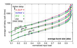
Fig. 9. Performance under varying average burst size (abs), for OQ, iSLIP with 4 iterations, buffered crossbar with 1-cell crosspoint buffers, and for the switch we propose in this paper with B=12, TH=5, and desynchronized clock credit schedulers: N=32.
