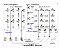
Fig. 2. The scheduling control unit of a VOQ switch with small, shared output queues; request, credit, and grant schedulers form a 3-stage pipeline, with request and grant counters being the pipelining registers.
