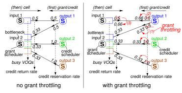
Fig. 4. An unbalanced transient with input 2 being congested. The busy (non-empty) VOQ shown are the ones shown; each busy VOQ corresponds to a busy request queue. The figure shows the credit reservation rates (assuming that credits are always available), and the credit return rates; (a) with no grant throttling, and (b) with grant throttling.
