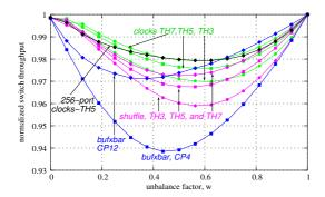
Fig. 8. Throughput under unbalanced traffic for varying threshold, TH, under different credit scheduling disciplines; B=12 cells; all switches have 32 ports, except one, 256-port clocks-TH5; Bernoulli arrivals.
