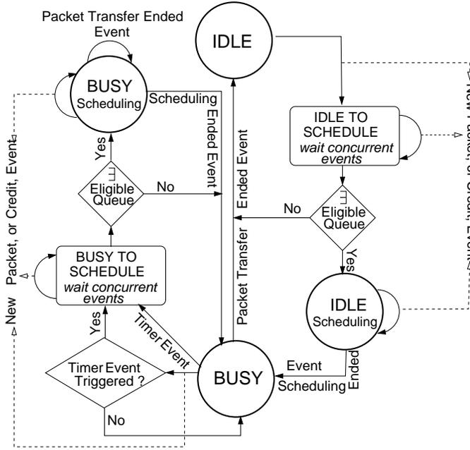
Fig. 14. Link/Scheduler Controller for Variable-Size-Packets
