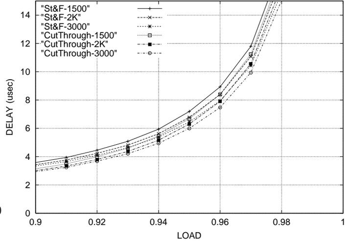
Fig. 11. Store&Forward Vs Cut-Through;  $32 \times 32$ , 10 Gb/s per port
