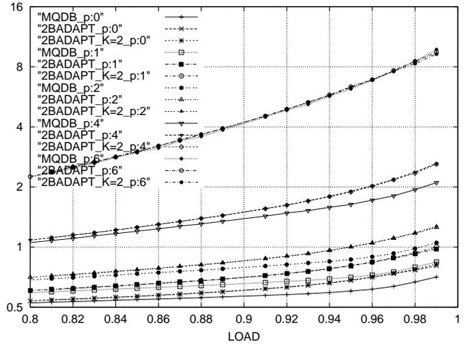
Fig. 29. 8 priority levels (p0 HIGHEST), **Poisson** arrivals. Y axis in logscale. 2B-ADAPT-K2 plots start at 0.8 load.
