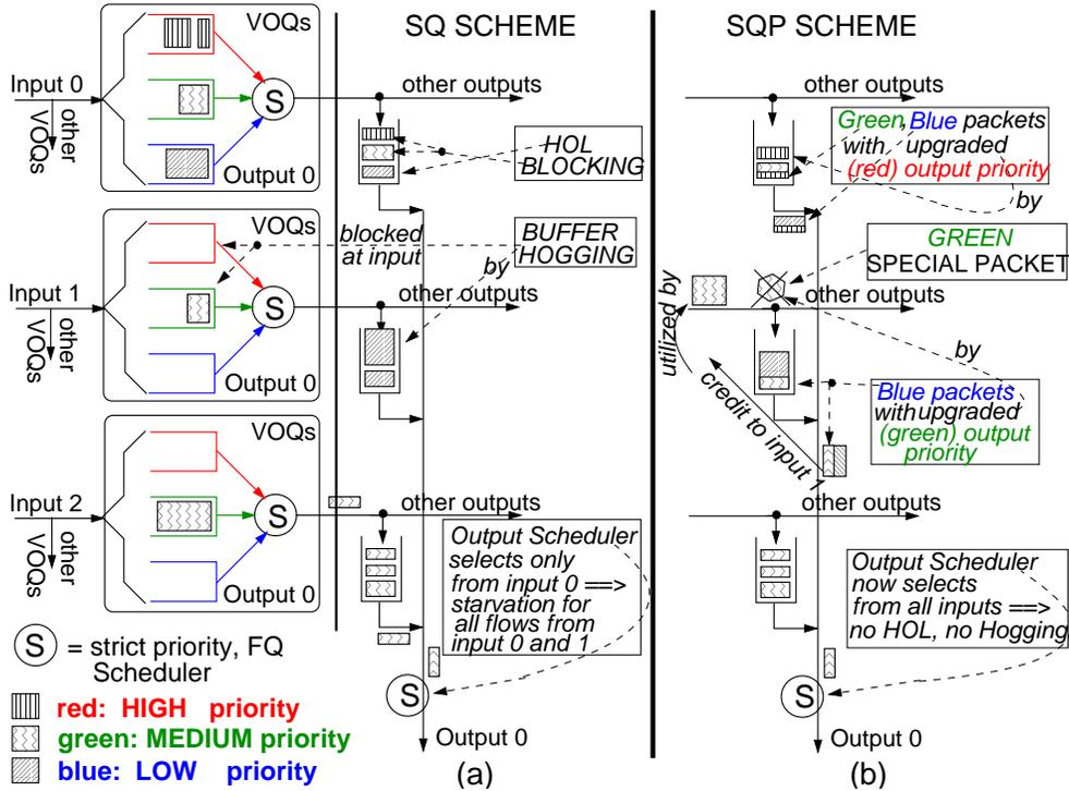
Fig. 16. (a) HOL blocking & Buffer Hogging in a SQ switch (b) SQP, see section 5.1.1
