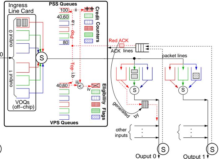
Fig. 7. A  $N \times 2$  buffered crossbar, supporting three priority levels with a separate crosspoint queue for each priority.
