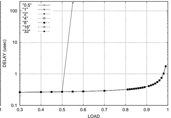
Fig. 4. 32×32 switch, 10 Gb/s port speed, 2 KByte buffer space per crosspoint; payload consists of MnPS packets only
