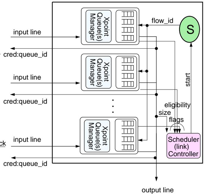
Fig. 39. The data-structures in an output controller.
