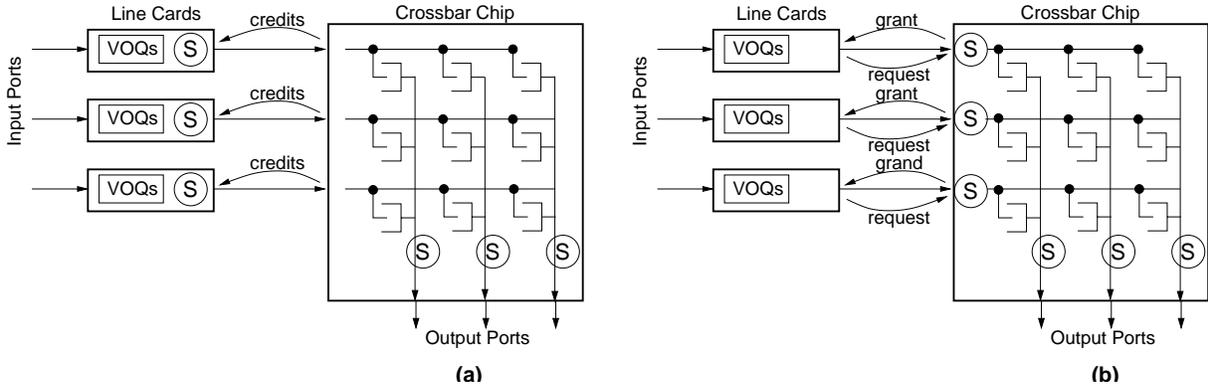
Fig. 5. A  $3 \times 3$  CICQ switch, (a) with the input schedulers at line-cards and (b) with input schedulers inside the crossbar chip
