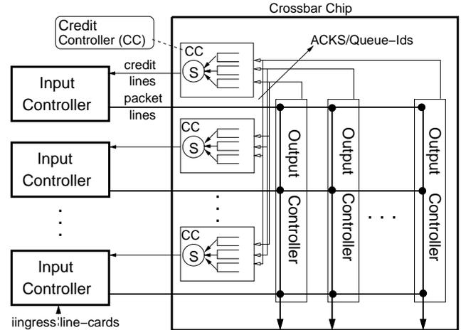
Fig. 37. The system controller; focus on the structure of the credit controller used in the simulation.
