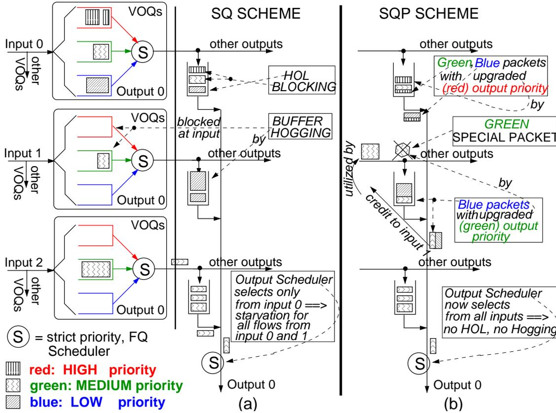
Fig. 15. (a) HOL blocking & Buffer Hogging in a SQ switch (b) SQP, see section 5.1.1
