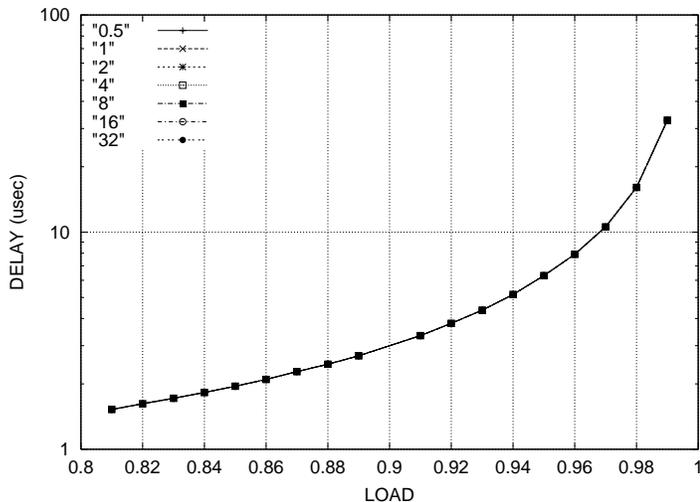
Fig. 3. 32×32 switch, 10 Gb/s port speed, 2 KByte buffer space per crosspoint; payload consists of packets with size that follows the Pareto distribution (average-packet-size 400 bytes, MnPS 40 bytes, MxPS 1500 bytes)
