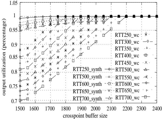
Fig. 10. RTT Experiment. For buffer size less than 1500 bytes, all measurements for output utilization are zero. Upper curves stand for SynthBackb traffic, lower curves for worst case.
