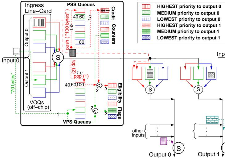
Fig. 6. A  $N \times 2$  buffered crossbar, supporting three priority levels with a separate crosspoint queue for each priority.
