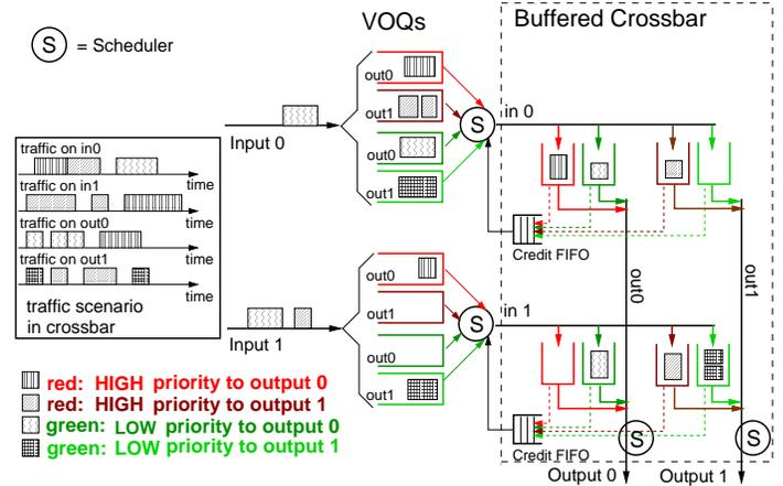
Fig. 2. A CICQ switch with a separate crosspoint lane for each priority level, i.e., the MQDB queuing organization –see section 4.1.1
