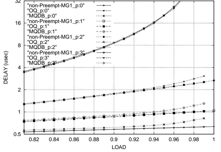
Fig. 20. 4 priority levels (p0 HIGHEST), **Poisson** arrivals. Y axis in logscale.
