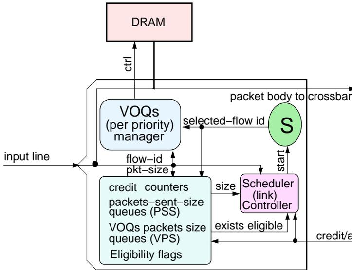
Fig. 38. The data structures in an input controller.
