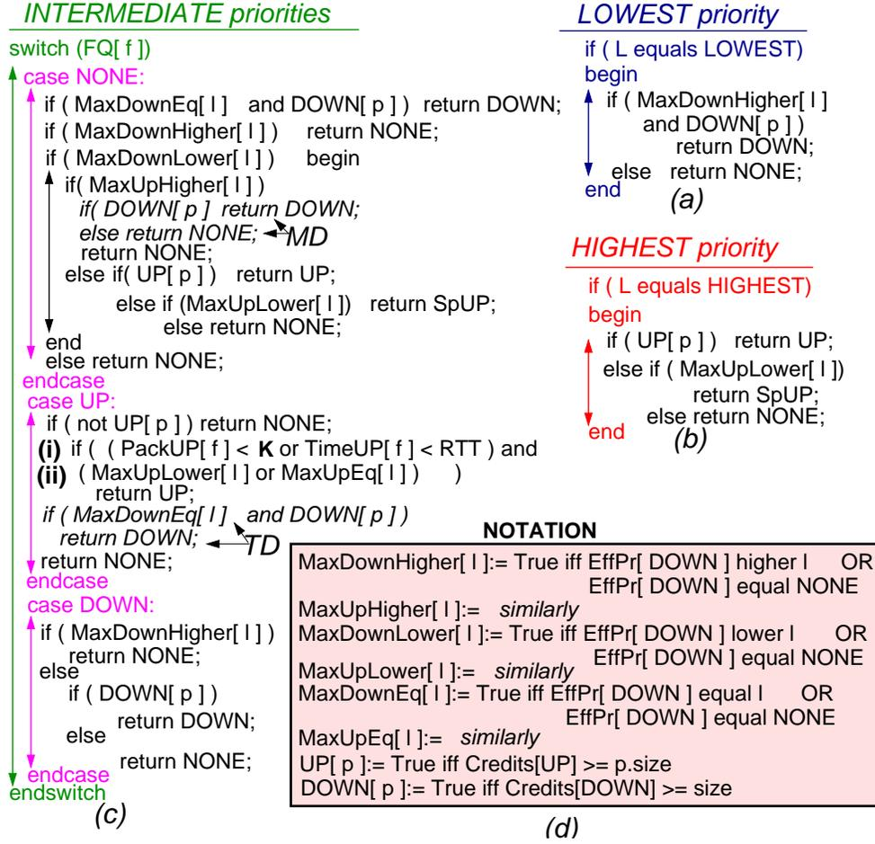
Fig. 18. Alg-2B-ADAPT policy for: (a) LOWEST priority; (b) HIGHEST priority; (c) Intermediate priorities. (d) Notation. (The lines in *italics* correspond to alternatives policies (i.e., TD and MD) and are *not* activated in 2B-ADAPT.)
