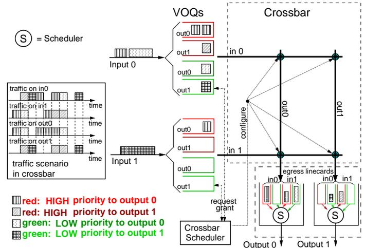
Fig. 1. The CIOQ switch with unbuffered crossbar
